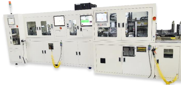
SOT-669 Trim from singulation system
